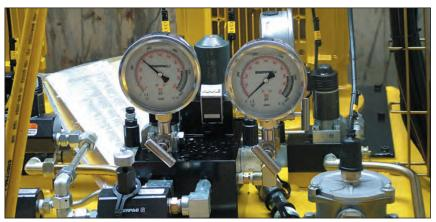
■ When lifting or pressing, always use a gauge. A gauge is your "window" to the system-it lets you see what's going on.
