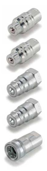
**5070-4, Male Tip.** Fits I-H 544788R1 and Pioneer 4057-4 female bodies. Ball style valving. Heat treated and zinc plated for resistance to wear and corrosion.
